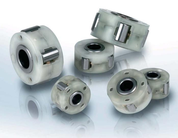
ype KI is a roller type freewheel. It is an assembly comprising of an inner race and rollers fitted into a polyamide cage. This type of unit can not be dismantled. It is designed for small mechanisms in office equipment, or packaging machines, to be mounted inside gears or feed rollers.
