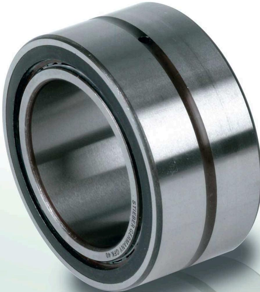
**T**ype GFK is a sprag type freewheel integrated into a 59.. series ball bearing. This design provides high torque capacity for minimal outside diameter. It is a bearing supported type, delivered grease lubricated.
