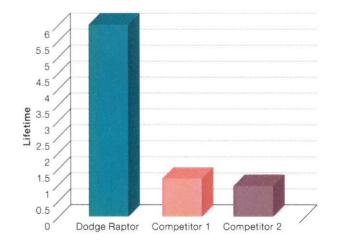
Results based on accelerated life testing at 1.5x catalogued torque, while subject to  $4^\circ$  angular misalignment and 4.8 mm parallel misalignment.
